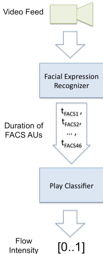
**Figure 1:** Overview of the automated play experience detector framework. The player's captured video is fed into the face recognizer which outputs FACS AUs[4]. These features are then input into the play classifier which determines the intensity of flow [13].
