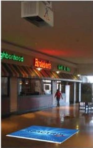
The box on the ceiling contains the video projector, IR LED lighting, the camera, and a wireless network client.
