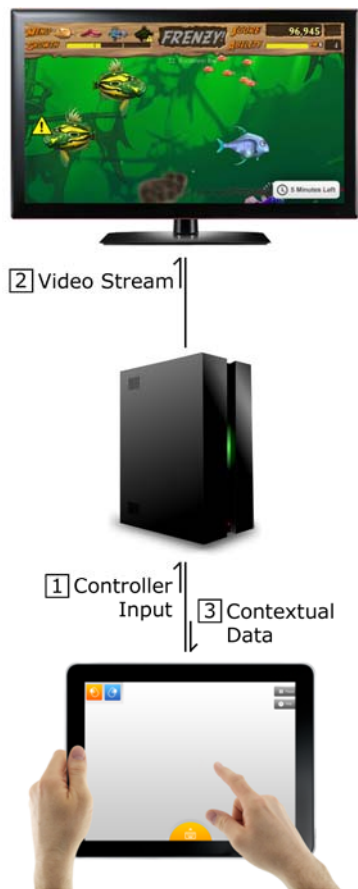
Figure 1: Project Blade creates a second-screen experience where a touch-screen device acts as a controller for a game being streamed to a television while the device receives contextual content from the streaming game related to gameplay.
