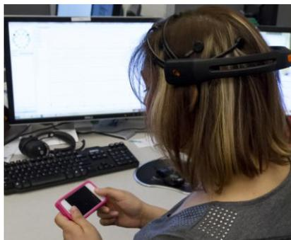
**Figure 1:** EPOC Emotiv Wireless EEG headset
